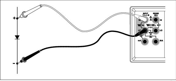
Figure 3-11. Diode Test
