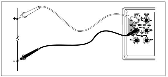
Figure 3-5. 2-Wire Resistance Measurement
