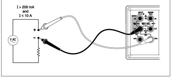
Figure 3-9. Current Measurement 200 mA to 10 A
