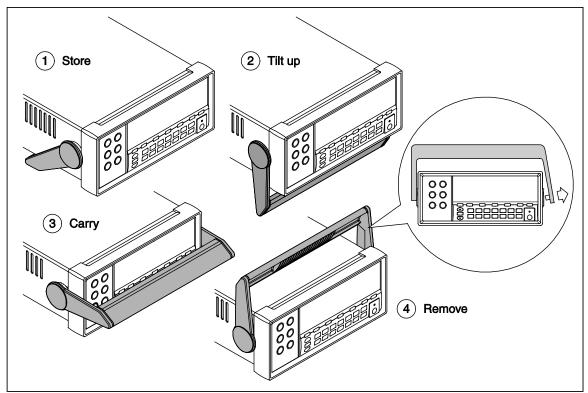
Figure 2-3. Bail Adjustment and Removal
