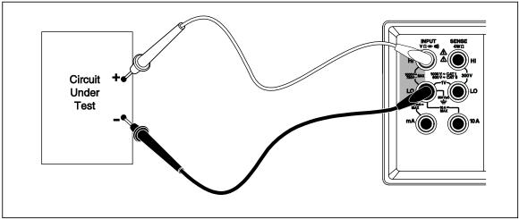
Figure 3-4. Voltage and Frequency Measurement
