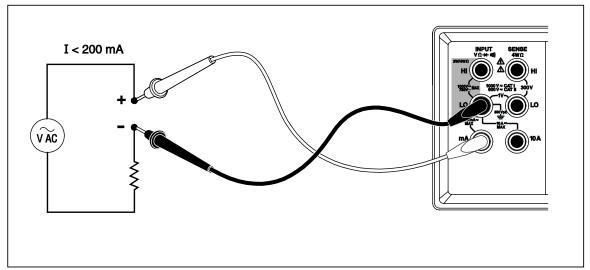
Figure 3-8. Current Measurement <200 mA
