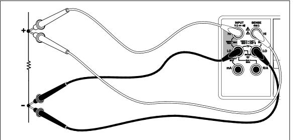
Figure 3-6. 4-Wire Resistance Measurement
