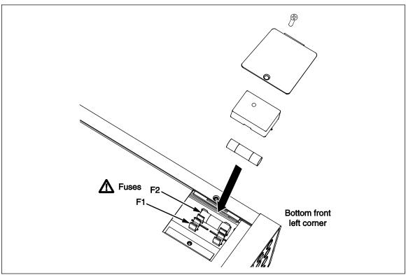
Figure 2-2. Replacing the Current-Input Fuses
