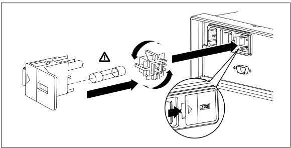
Figure 2-1. Replacing the Line Power Fuse
