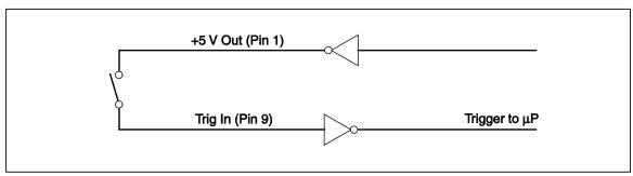
Figure 3-12. External Trigger Circuit
